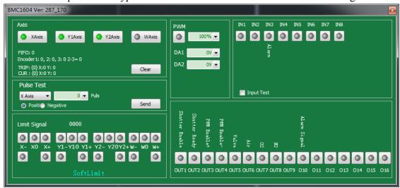
Please check in sequence positive/negative/origin switch of each axis, input signal, output signal, DA signal, PWM signal and servo-enabled signal.
