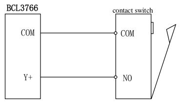
Typical connection of magnetic switch is shown as below, which must use 24V switch of the NPN type.
