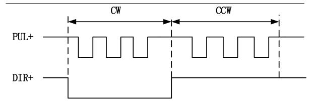
The output way of differential signal is shown as below:
