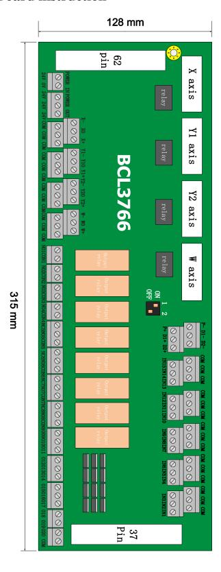
The External IO Board of BCL3766 is installed by rail and also can be installed permanently. Its external size is 315mm\*128mm with DM62M and DB37M interface in two sides, corresponding to JP1 and JP2 of BMC1604V2. C62-2 cable is used to connect External IO Board DB62 interface with JP1 port on the back of control card JP2 interface is linked by C37-40 baffle wire and then is fixed on erection fixture of computer with bolts. And C37-2 cable is used to connect DB37 socket on External IO Board.
