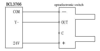
Typical connection of contact switch is shown as below: •
